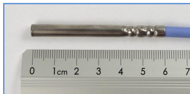
Fig. 3 – Temperature sensor for THT2
